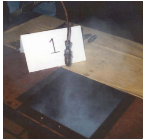
Spray pattern testing on injection nozzle 1 of SDN 982 vehicle
