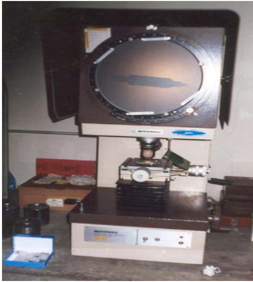
Full view of injection nozzle pin projected by the profile projector equipment
