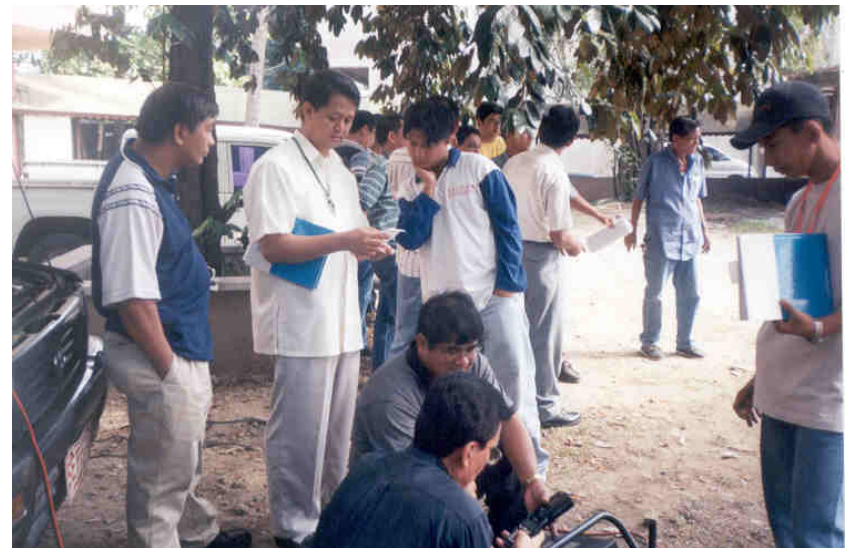
SMOKE EMISSION TESTING OF PCA VEHICLE (MITSUBISHI L-200) ON JANUARY 10, 2002 BY DENR TECHNICIAN. CHECKING THE "k" OR OPACITY PRINTOUT DATA RESULTS
