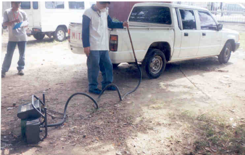
SMOKE EMISSION TESTING OF PCA VEHICLE (MITSUBISHI L-200) ON JANUARY 10, 2002 BY DENR TECHNICIAN. CHECKING THE "k" OR OPACITY PRINTOUT DATA RESULTS
