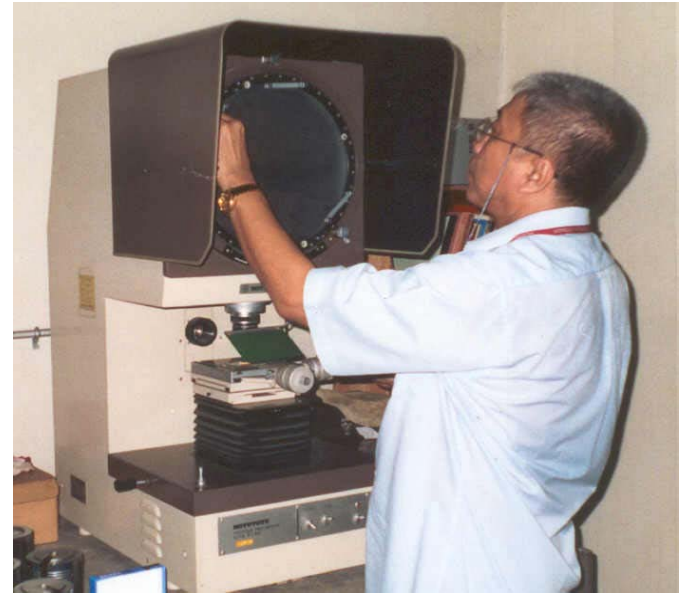
Professor Loreto G. Aguila preparing the Profile Projector equipment to measure the injection nozzle tiny parts.
